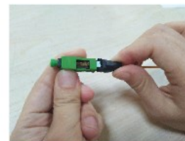
9. Screw down the boot along the thread
