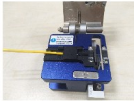
7. Pull the yellow button to lock the fiber
