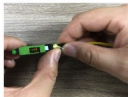
8. Rotate the aramid yarn along the thread
