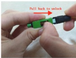
10. Pull the yellow button to unlock the fiber
